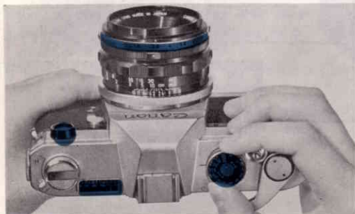
5. Determine the exposure with built-in meter.
